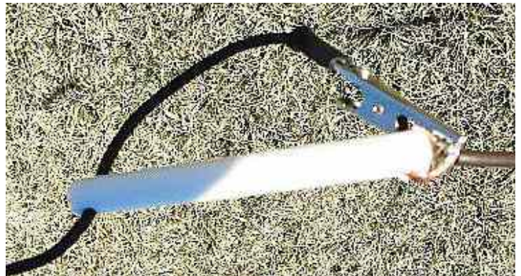
Connected alligator clamp to counterpoise
