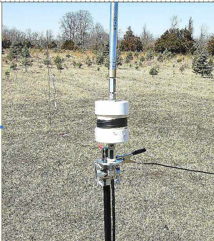
40-meter coil with antenna clamp, counterpoise connection to clamp and one counterpoise
